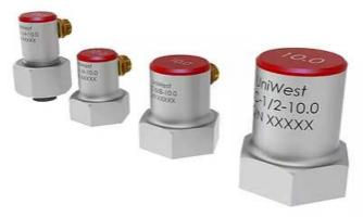
Single element compression wave transducers are generally used for applications such as flaw detection, metal thickness estimation and feature mapping. The Standard Contact configurations are housed in a rugged stainless-steel shell couple with an aluminium oxide wear face. Replaceable delay
