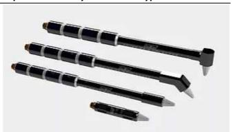
Replaceable delay line pencil type transducers are produced with a single crystal element and rugged design, making them perfect for tough work settings. The special design allow testing to be completed in difficult to access areas of work pieces. They have great sensitivity and second to none resolution. The tips are replaceable and come with diameters 1.8, 2.3, and 3.2mm.
